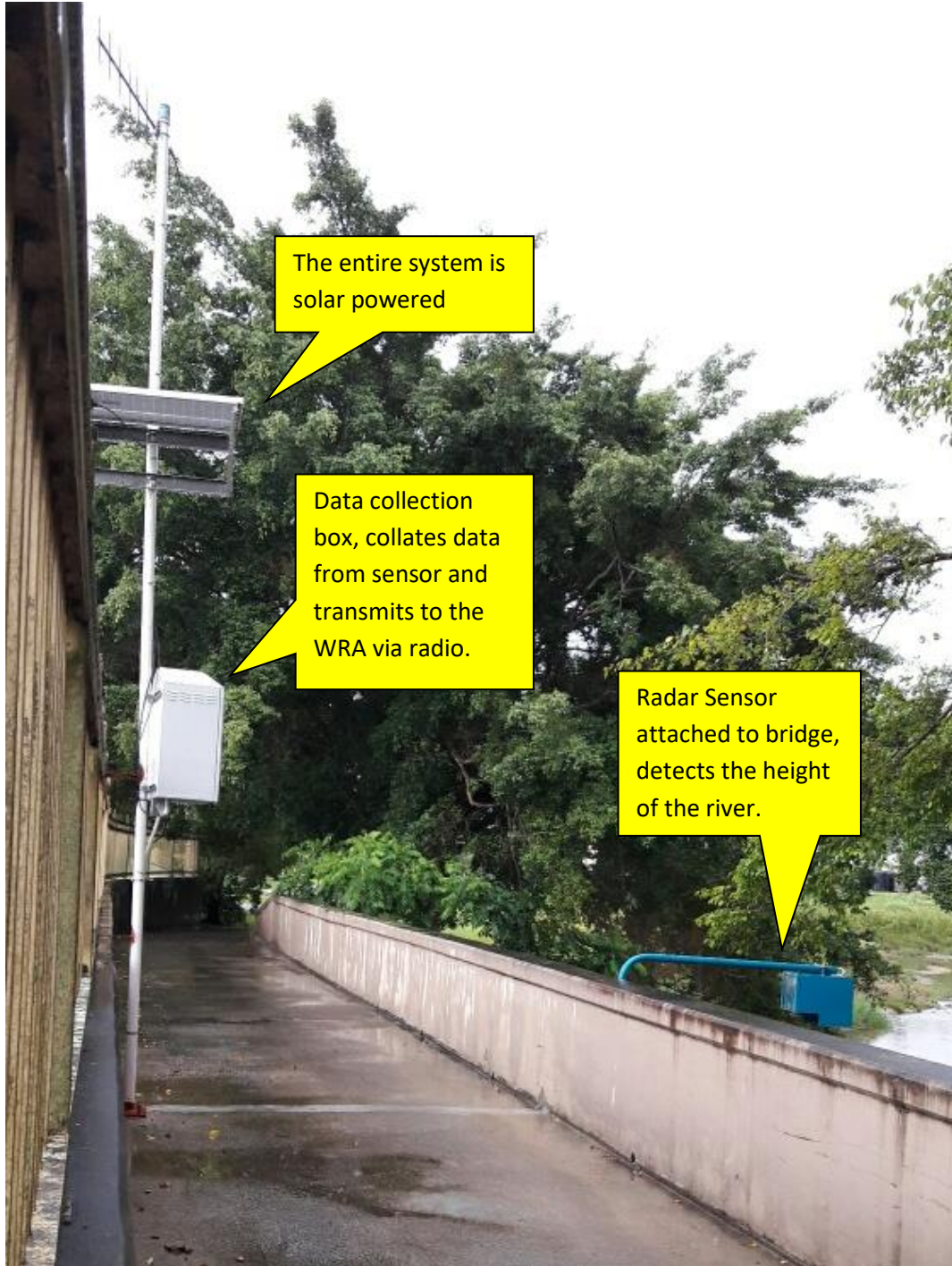
Figure 2: Arouca Streamflow Station located on a bridge over the Arouca River. This streamflow station will provide early warning to the communities of Oropune and part of St. Helena.
